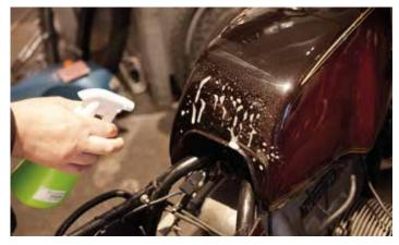
**1** Mix tap water with a little commercial washing-up liquid and spray the area of the tank to be painted.
