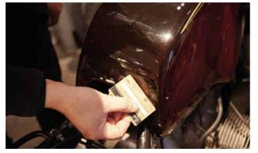
**6** When the film has been positioned correctly, use a cheque card or similar (e.g. dough scraper) to wipe out the water. If necessary, smooth out air bubbles with your fingers towards the edges. Any remaining moisture diffuses through the film so that it disappears completely.
