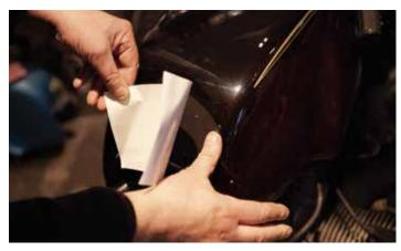
**4** Peel off about half of the backing paper and press the film onto the tank. Then hold the detached side of the film and remove the backing paper completely.
