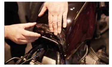
**5** The film can be moved as long as the liquid is still present and positioned exactly. Do not touch the adhesive side, otherwise fingerprints may remain on the adhesive.
